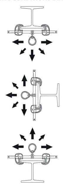
Placement at or below a user's working height requires integration of a compatible ANSI Z359.1 shock-absorbing lanyard that does not allow the user to extend more than 6 feet (in any direction) from the anchorage connector before the shock absorber is activated. The beam anchor must be attached to the I-beam flange facing the user (top flange if above, bottom flange if below, etc.).
